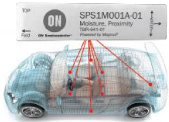
Figure 3: Sensors are placed directly on the vehicles' metal chassis at the pre-trim stage
