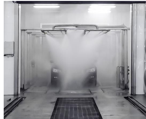
Figure 1. Automakers turn up the pressure to find leaks with water jets in the 2,000 psi range
