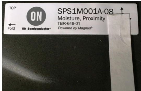
Figure 4: Wireless moisture sensor installed on bare chassis metal with optional wicking tail that extends the monitoring zone
